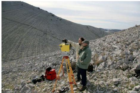
FIG 2: Optech 36D long range laser 3D scanner coupled with GPS/GLONASS receiver Topcon HIPER+ (Plus) GNSS
